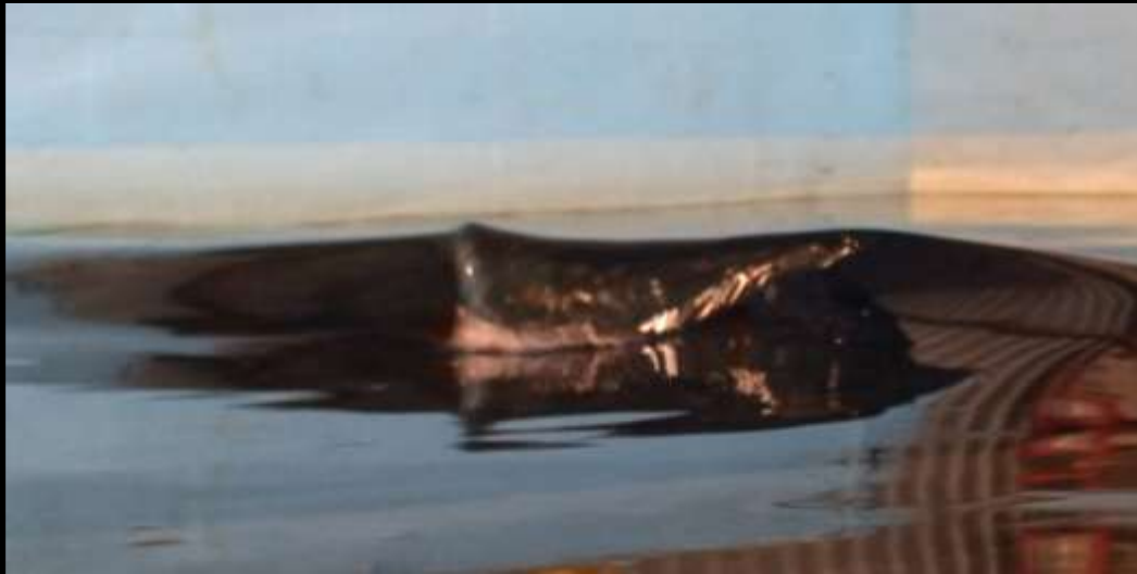
Wave Breaking on Laboratory Model
